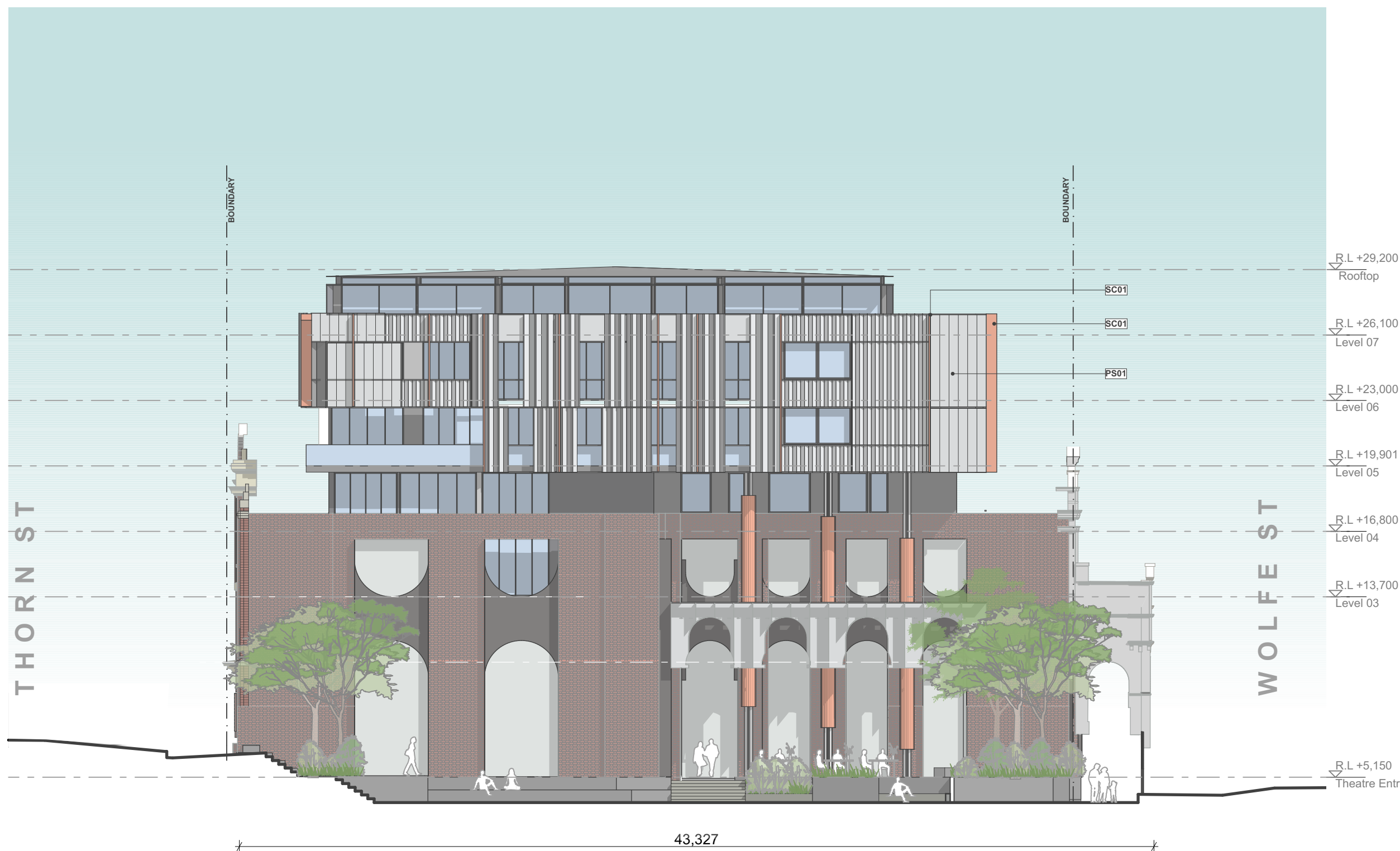
LANEWAY (SOUTH) ELEVATION SCALE 1:200 @ A1
